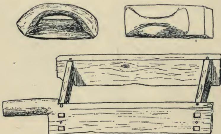
89. PLASTERERS' FLOATS, AND BRICK-MOULD.
